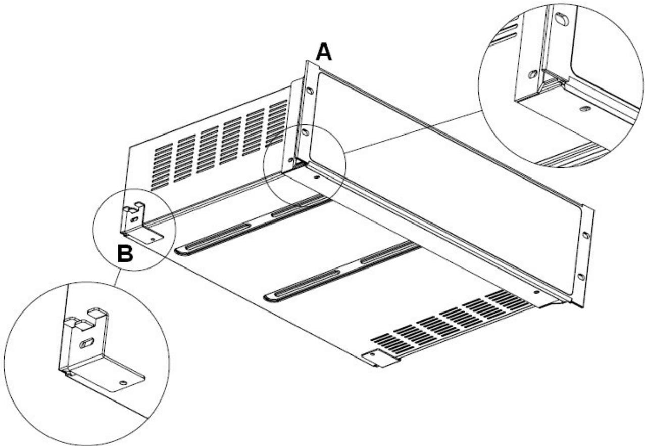
**1** Remove the four rubber feet from the amplifier bottom.
