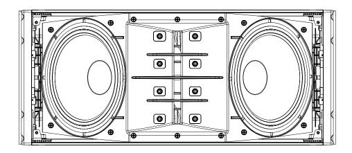
The custom-designed waveguide allows a precise coverage of 100 x 15 degrees, whilst also delivering a superb linear HF response.
