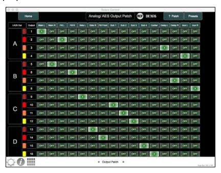
Figure 15: Analog/ AES output patch
