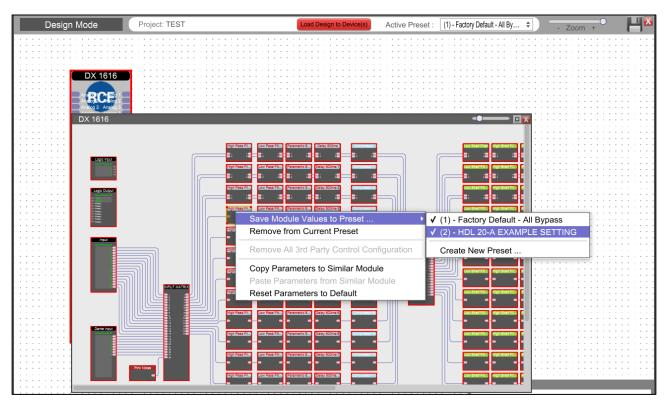
Figure 27: "Design Mode" – Save Module Values to Preset
