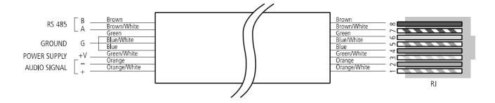
Correspondence of wires between CAT 6 and CJ 428CAT cables:
