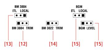
[12] **BM 3804 TRIM** jumper: BM 3804 [1] audio input gain setting, useful to compensate for possible signal attenuation along the line.
