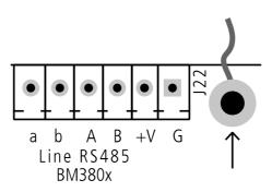
DESCRIPTION PIN **BM 3022 CABLE – WIRE COLOUR** Audio signal (+, hot) Orange/White (RJ pin 1) +Audio signal (-, cold) Orange (RJ pin 2) \_ G Ground (audio) Blue (RJ pin 4) Priority and activation command Green (RJ pin 6) Pq G Priority and activation command ground Green/White (RJ pin 3)
