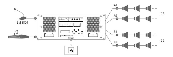
On request, the main unit can be delivered with four (MXR 4500/4) / six (MXR 4500/6) built-in power amplifiers.
