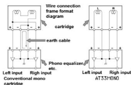
The AT33Mono is made specifically for use on mono systems. It has a horizontal coil, and so in principle only generates electricity horizontally.
