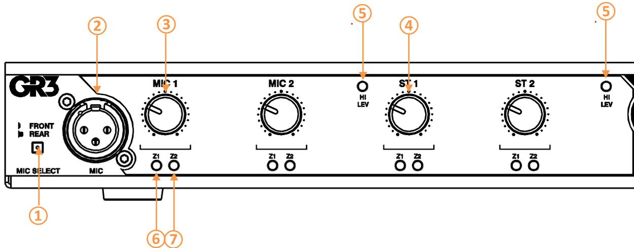
**① MIC SELECT** – a user selectable switch for MIC 1 input. MIC 1 signal can either be derived from the rear mount Euroblock or front mount XLR connectors. Use pointed object to select switch.
