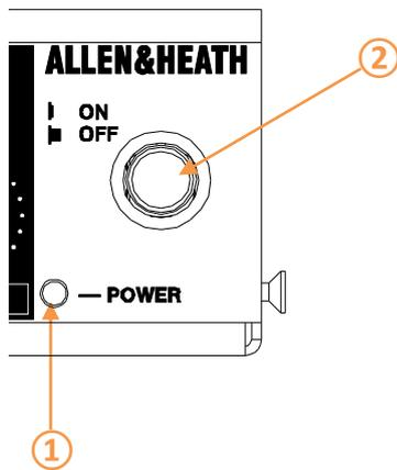
① **POWER INDICATOR** – LED indicator showing the unit has power. Also used to indicate when unit is in 'Programming' mode (see section 6.4).
