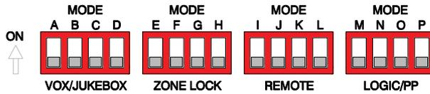
**DIP switch settings** Up = ON. Factory default = all switches down (OFF).
