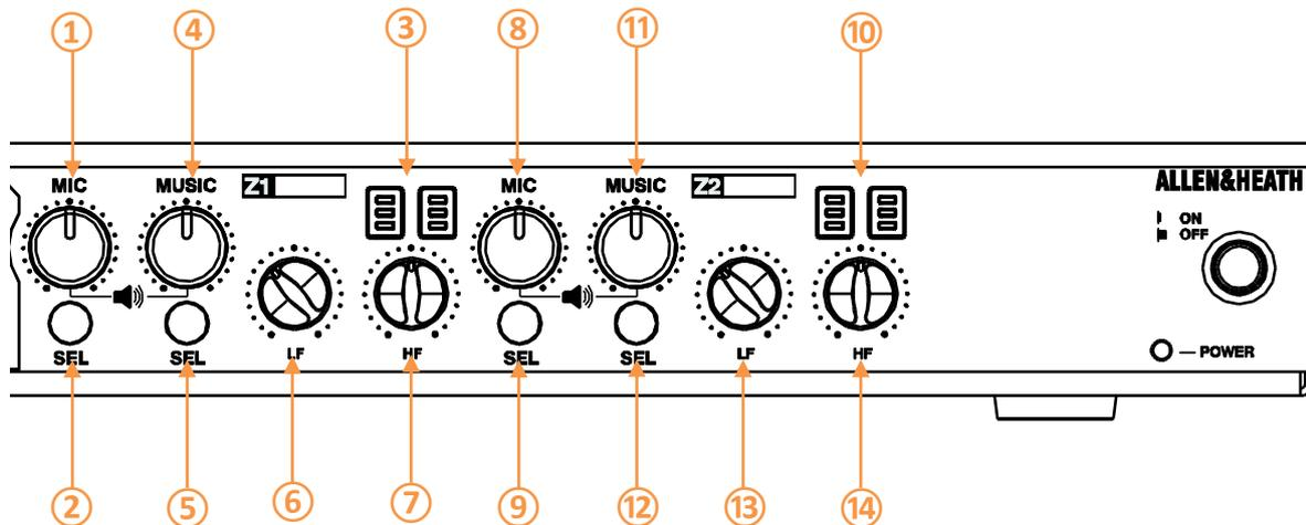
**① Z1 MIC MIX OUTPUT LEVEL** – Adjustable rotary level control for MIC Mix to Zone 1. Output level control Off to +6dB.
