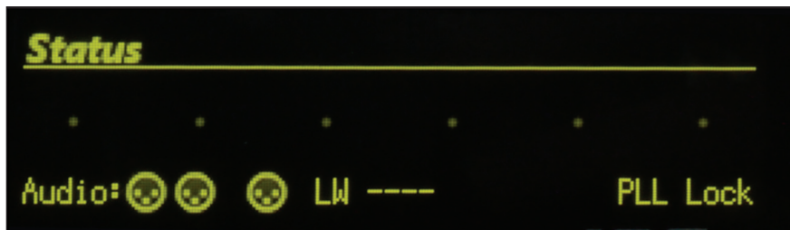
Typical status screen for traditional I/O connections
