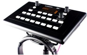
**ME-1** is a stand-alone digital personal mixer receiving up to 40 sources via a single Cat5 cable from the main console and mixing these to a stereo and mono output to drive headphones, in-ears, loudspeakers or other monitoring devices.
