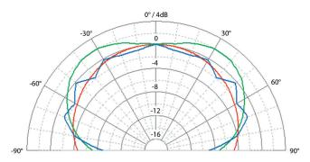
SC407, horizontal configuration: Polar pattern (1m): 200Hz / 1kHz / 5kHz
