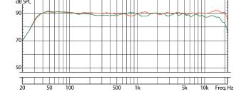
SC408, horizontal configuration: Free-field frequency response (1/6 oct.): 0° / 30° horizontal off-axis
