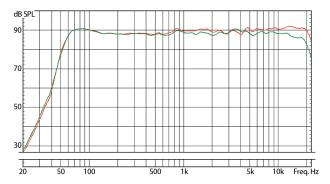
SC205: Free-field frequency response (1/6 oct.): 0° / 30° horizontal off-axis
