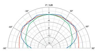
SC407, vertical configuration: Polar pattern (1m): 200Hz / 1kHz / 5kHz
