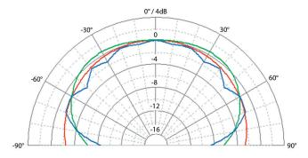
SC3012, vertical configuration: Polar pattern (1m): 200Hz / 1kHz / 5kHz
