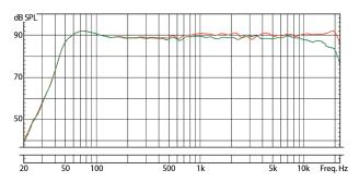
SC207: Free-field frequency response (1/6 oct.): 0° / 30° horizontal off-axis
