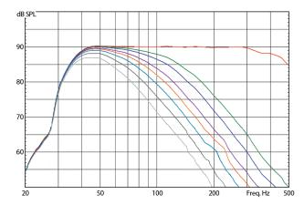
TS107: Free-field frequency response (1/6 oct.): LFE + different filter settings down to 60Hz
