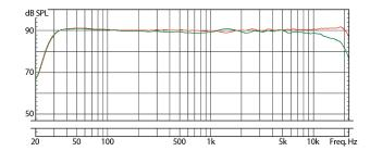
SC3010, vertical configuration: Free-field frequency response (1/6 oct.): 0° / 30° horizontal off-axis
