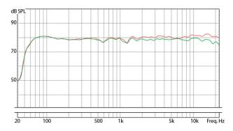
SC203: Free-field frequency response (1/6 oct.): 0° / 30° horizontal off-axis
