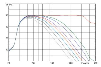
TS108: Free-field frequency response (1/6 oct.): LFE + different filter settings down to 60Hz
