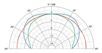
SC204: Polar pattern (1m): 200Hz / 1kHz / 5kHz
