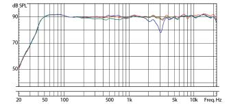
SC307, horizontal placement: Free-field frequency response (1/6 oct.): -15° / 0° / +15° horizontal off-axis
