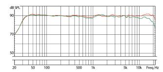
SC408, vertical configuration: Free-field frequency response (1/6 oct.): 0° / 30° horizontal off-axis
