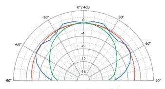
SC208: Polar pattern (1m): 200Hz / 1kHz / 5kHz
