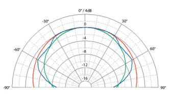
SC408, vertical configuration: Polar pattern (1m): 200Hz / 1kHz / 5kHz
