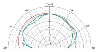
SC3010, horizontal configuration: Polar pattern (1m): 200Hz / 1kHz / 5kHz
