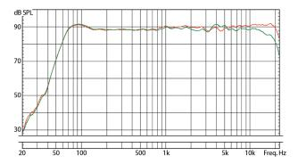
SC204: Free-field frequency response (1/6 oct.): 0° / 30° horizontal off-axis
