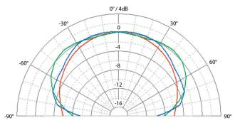
SC408, horizontal configuration: Polar pattern (1m): 200Hz / 1kHz / 5kHz
