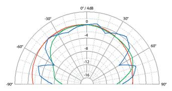
SC307, horizontal placement: Polar pattern (1m): 200Hz / 1kHz / 5kHz
