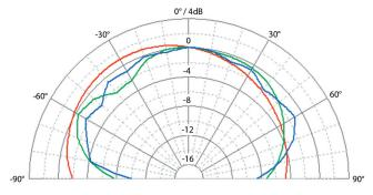
SC3012, horizontal configuration: Polar pattern (1m): 200Hz / 1kHz / 5kHz
