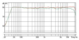
SC208: Free-field frequency response (1/6 oct.): 0° / 30° horizontal off-axis
