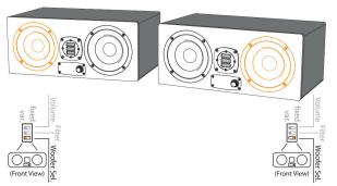
With the SC305/SC307 placed vertically, the rear Woofer Sel. switch should be set differently depending on the listening position:
