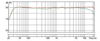
SC3010, horizontal configuration: Free-field frequency response (1/6 oct.): 0° / 30° horizontal off-axis
