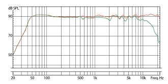
SC307, vertical placement: Free-field frequency response (1/6 oct.): 0° / 30° horizontal off-axis
