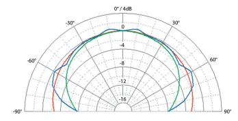
SC3010, vertical configuration: Polar pattern (1m): 200Hz / 1kHz / 5kHz
