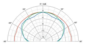
SC205: Polar pattern (1m): 200Hz / 1kHz / 5kHz
