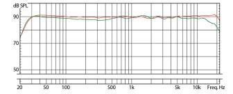
SC3012, horizontal configuration: Free-field frequency response (1/6 oct.): 0° / 30° horizontal off-axis
