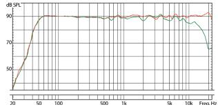
SC305, vertical placement: Free-field frequency response (1/6 oct.): 0° / 30° horizontal off-axis
