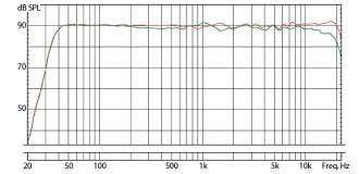
SC407, horizontal configuration: Free-field frequency response (1/6 oct.): 0° / 30° horizontal off-axis
