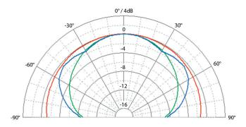
SC207: Polar pattern (1m): 200Hz / 1kHz / 5kHz
