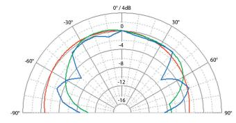
SC305, horizontal placement: Polar pattern (1m): 200Hz / 1kHz / 5kHz
