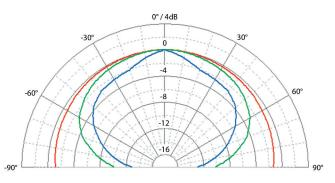
SC305, verticalal placement: Polar pattern (1m): 200Hz / 1kHz / 5kHz
