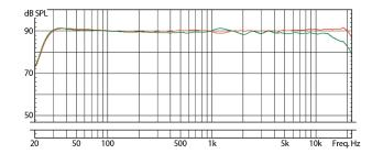
SC3012, vertical configuration: Free-field frequency response (1/6 oct.): 0° / 30° horizontal off-axis
