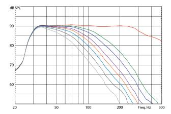
TS110: Free-field frequency response (1/6 oct.): LFE + different filter settings down to 60Hz
