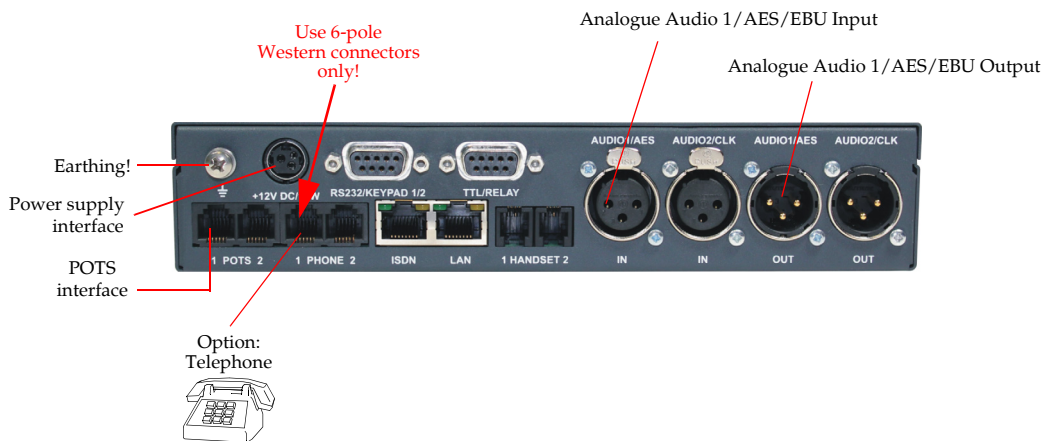
FIG. 4 MINIMUM WIRING IN POTS OPERATING MODE
