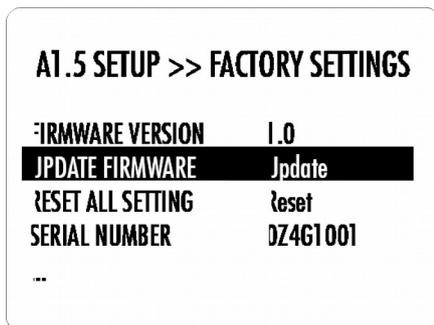
The A1.5 SETUP >> FACTORY SETTINGS menu allows to get information about current A1.5 firmware version, to update the A1.5 firmware and to reset the unit to default configuration (or subset of settings).
