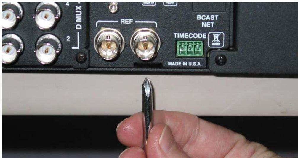
3. Pull the monitor so that it slightly hangs over the edge of the surface on which it is sitting, and remove the screw on the bottom as shown in Figure 6-12 above.
