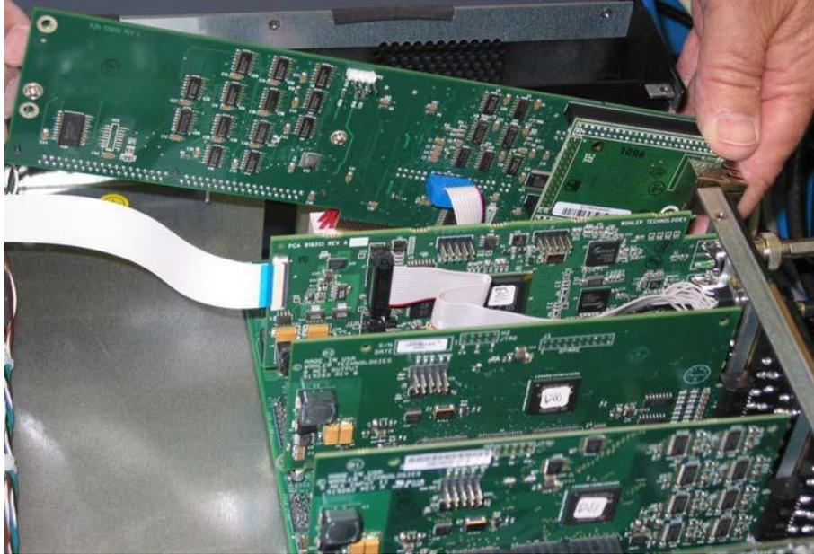
14. Firmly press the system control board back into its slot so that it is securely connected as shown in [Figure 6-22](#). Generally, this board does not snap in.
