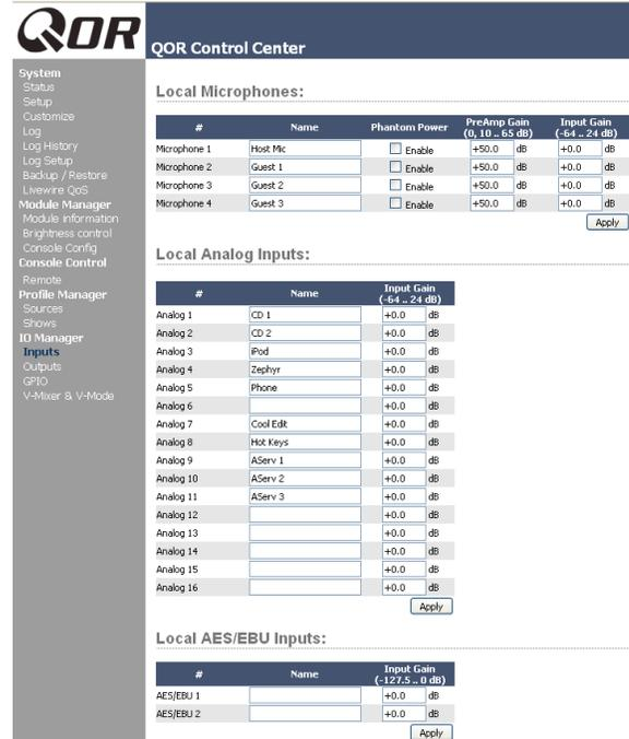
Figure 2-1: Audio IO Manager - Inputs from QOR.32
