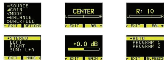
When viewing these menus, the **Options** control is pressed to select the function, and rotated to set
