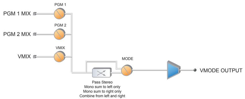
Figure B-6 Block Diagram - Master Output
