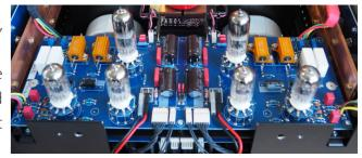
Like the entire InPoL Legacy structure, the tube power supply is separate, with a toroidal transformer for each channel.
