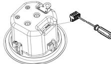
5. Use the provided loop-through terminals (see graphic below). When this wiring method is used, you should be aware that when a speaker is not plugged in there is no path to subsequent speakers. An alternative is to wire incoming and outgoing cables in parallel. Pin 2 is + and Pin 3 is - (see graphics below).
