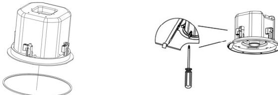
8. Use a flat-head screwdriver to rotate the Tap Selector so that the correct power setting is adjacent to the arrow. Note that there are separate 70V and 100V scales, depending on the line voltage being used (see the graphic below). The transformer may also be bypassed by selecting the 16 ohm position. It may be best to leave the grill off until the setting of the power is complete in case adjustments are needed.
