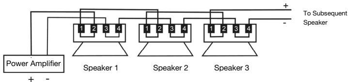
6. Insert the pre-wired Euroblock connector, ensuring the correct polarity is being used.
