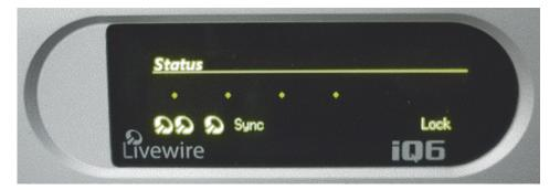
The status screen provides the state of each of the six telco lines (states are indicated by icons described in chapter 3), input state, digital sync, and lock.
