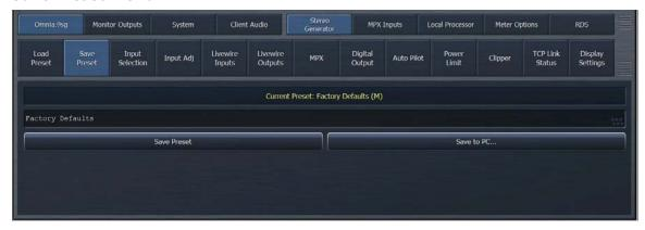
This is where you can save any customizations or changes you've made to the controls in the "Stereo Generator" section.
