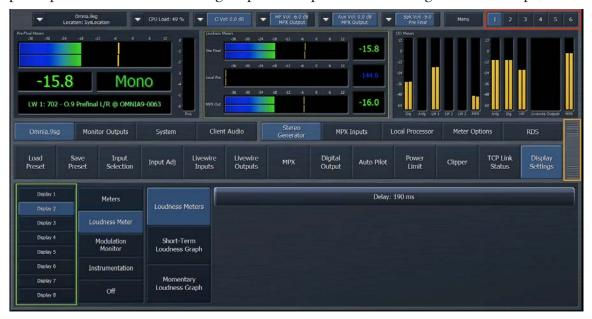
A row of six "Display Preset" buttons is located at the top right corner of the NfRemote display, outlined here in red. Each display preset can show up to eight display windows, outlined here in green. The number of simultaneous displays used in each preset will depend primarily upon monitor size as adding displays reduces the size of each individual window and will, on smaller monitors, quickly make them less readable and useful.
