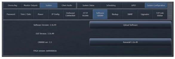
The "Software Update" menu displays the current 9sg software (and NfRemote client) version as well as the versions associated with several internal 9sg components.
