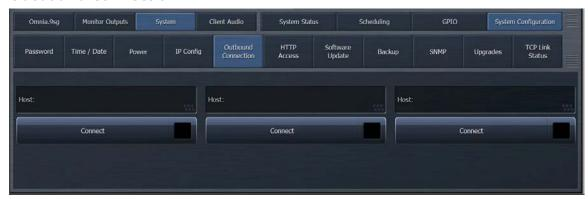
While the most common mechanism for connecting NfRemote to Omnia.9sg is via an IN-BOUND connection initiated from the remote client, in some cases (such as certain firewall restrictions) it may be more useful for the 9sg to initiate the connection to one or more remote clients.
