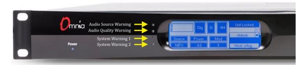
The top two LEDs denote audio conditions and alarms, the "Audio Source Warning" and "Audio Quality Warning" indicators. The bottom two are system status and alert indicators, "System Warning 1" and "System Warning 2".
