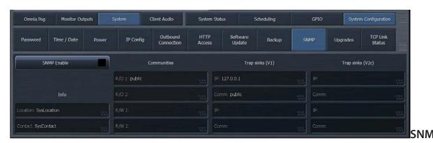
The SNMP menu provides the means to enter the information necessary to facilitate communication between Omnia.9sg and your SNMP manager. It supports SNMP V1 and V2c.
