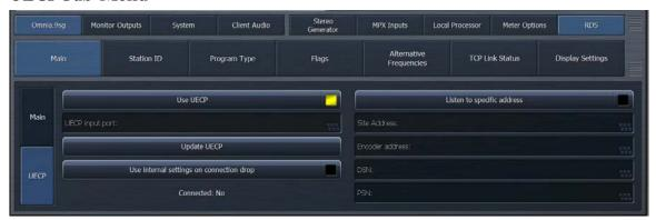
UECP (Universal Encoder Communications Protocol) is a standardized protocol for communicating with RDS encoders and provides the ability to address all encoders, specific groups of encoders, or individual encoders. This is particularly useful in non-U.S. applications where the use of RDS is more highly developed and embraced and where identical content is broadcast from multiple geographically-diverse transmitter sites.
