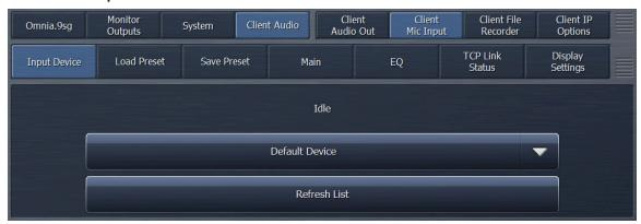
The Client Microphone Input Menu allows you to pick which microphone you'd like to use, a parametric equalizer to create custom EQ curves for individual mics, and the ability to save and recall custom mic presets.
