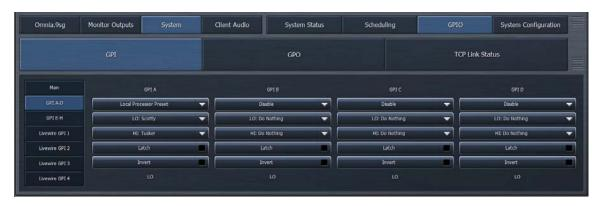
GPI functionality is enabled or disabled in the "Main" tab. Please note that GPI must be disabled in order to make any GPI configuration changes.
