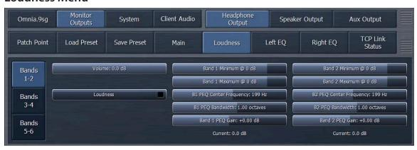
The audio monitoring tools in 9sg also include a loudness curve adjustment. These controls (much like the "Volume-Based High Pass Filter" mentioned earlier) can compensate for monitoring systems with an uneven frequency response that varies based on the volume. There are 6 bands of control available (displayed in groups of 2) and all function identically.
