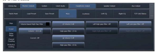
The "Main Menu" contains controls that allow high-pass and low-pass filter frequencies to be set and also permit different high pass filtering depending upon the setting of the "Volume" control. This can compensate for systems that have an uneven frequency boost applied to make them sound better at low volumes which does not scale appropriately with increased volume.
