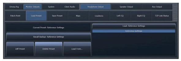
Because Omnia.9sg (along with the "Client Audio" feature built into NfRemote) provides all of the tools – minus a calibrated microphone – to perform speaker/room calibrations for each Monitor Output, it also provides a means by which to store those calibrations for later recall in the form of presets.
