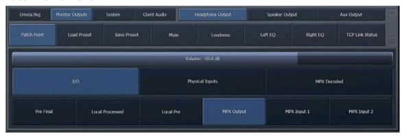
Three audio input sources are presented here – "I/O", "Physical Inputs", and "MPX Decoded".
