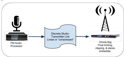
Some FM broadcasters are transmitting the same audio from two or more tower sites. In these cases, one primary audio processor can feed a WAN or satellite distribution system while individual Omnia.9sg's reside at each transmission site.
