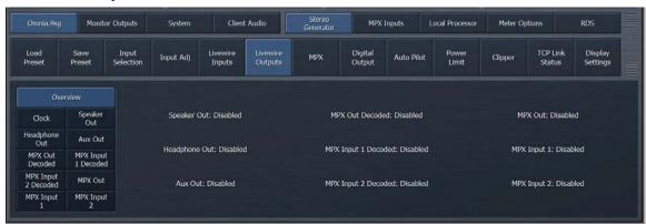
Multiple Livewire outputs from various paths within the Omnia 9.sg can be generated and sent to the network. The Overview screen will allow you to see what Livewire channels are currently being generated, and from which source or path within the unit the channel will contain.
