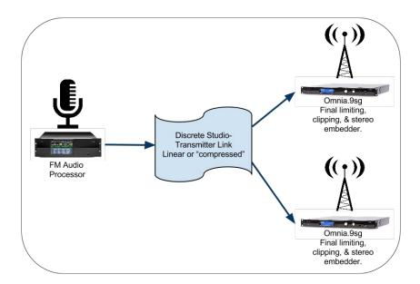
Transmitter sites are often remotely located and sometimes shared among multiple broadcasters. Access may be limited and tightly controlled. In such cases, keeping the main processor at the studio and installing a smaller and less expensive stereo encoder makes sense.
