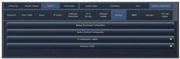
This menu allows a full backup and restore of the 9sg configuration. Although an update will normally not affect the unit's configuration, it is a good idea to backup your configuration prior to performing a software update.
