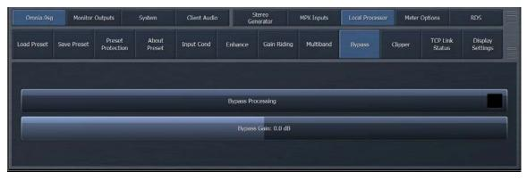
Enabling the "Bypass Processing" button bypasses all dynamics processing. The "Bypass Gain" control should be set so that the level of unprocessed (bypassed) audio matches the average level of process audio as closely as possible.
