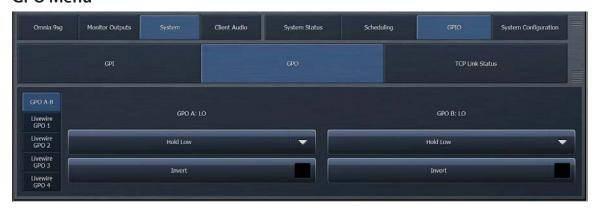
Available GPO functions can be selected from the "Hold Low" drop down menu and include several critical status or alarm conditions as well as a logical GPI echo, physical GPI echo, plus half- and quarter-Hz test signals. All GPOs will hold until the alarm situation passes and normal status resumes. By default, "Low" is considered the alarm condition (while "High" is a normal status) but this can be flipped by checking the "Invert" control.
