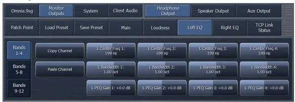
Following the main monitor controls (x-over, delay/phase, loudness) is another fully parametric EQ for "fixed" frequency response tuning of the monitor system, not based on the monitor volume level. There are 12 bands of EQ available (displayed in groups of 4).
