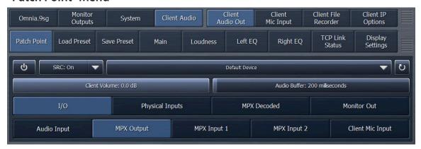
To enable client audio output, click the "power button" icon in this menu. A selectable Sample Rate Converter (SRC) ensures that the audio remains stable, though when enabled this feature consumes additional CPU resources.
