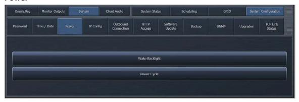
Allows a "clean" remote power cycle of 9sg. Normally this would only be necessary for troubleshooting purposes. Use this with caution as it WILL (obviously) take the 9sg off the air as it reboots. If you have an external processor connected to the MPX input, the internal relay bypass should pass signal from that audio processor through to the MPX output while the 9sg reboots. You can also "wake up" the front panel backlight remotely from this menu.
