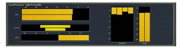
• The "I/O Meters" display shows the levels of all input audio sources and all physical outputs.
