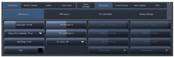
Omnia.9sg offers two rear panel composite (MPX) inputs which can be used to feed the output of an external RDS generator, the composite output of another processor, or the composite output of a tuner or frequency-agile modulation monitor.
