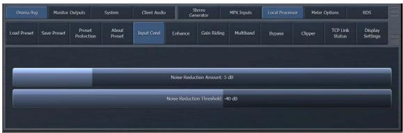
The "Input Conditioning" menu contains the controls for the multiband downward expanders which can be helpful for managing noisy content (such as tape hiss on old recordings) or environmental noise (such as HVAC noise).
