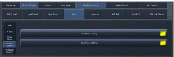
In some installations, the left and right speakers are in similar locations within the room and relative to the monitoring point. In these situations, EQ and Delay settings can be applied to both channels by enabling the "Common L/R EQ" and "Common L/R Delay" controls.
