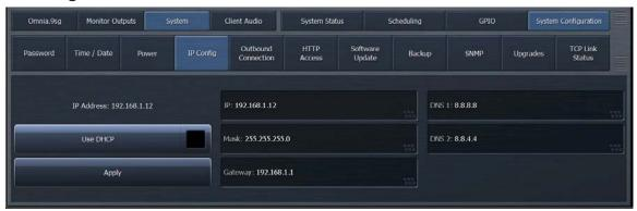
This menu allows configuration of the unit's IP address, subnet mask, gateway, and DNS servers. It also allows you to select configuration via DHCP. The currently assigned IP address is one of the first items displayed in this menu.
