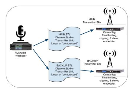
Research has indicated that ratings encoders and/or ratings enhancement devices (such as our own Voltair) benefit from being fed processed audio. While some processors including Omnia.9 and Omnia.11 have special "insert points" designed for this purpose, not all processors do. Placing the processor and ratings encoder at the studio and moving the stereo generator to the transmitter site can help accommodate this.
