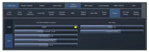
These controls affect the texture and feel of the bass clipper and are sub-divided into two groups: "Bass Intermodulation Protection" and "Bass Shape"
