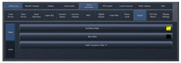
The clipper menu contains controls that allow the sound and texture of the clipper to be fine tuned. Please remember that the overall clipper drive is determined by the "Input Gain" control in the "Input Adjust" menu.
