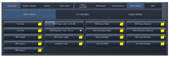
Exactly which meters appear in the Loudness Meter, Modulation Meter, and Modulation Numeric display windows is determined by enabling or disabling various options in this menu. If you do not see a meter you expect to see in any of the graphs or meters, check this menu to ensure the one you are looking for has been enabled.
