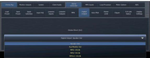
The source feeding the rear panel AES Digital Output is set here and includes Omnia Direct, which allows a composite signal from Omnia.9sg to be carried on a single AES-EBU cable connection between the stereo generator and an Omnia Direct-enabled transmitter.
