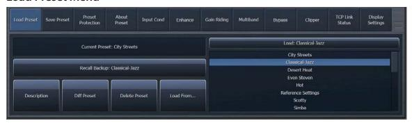
The "Load Preset" menu allows you view the preset currently on the air, toggle back and forth between the current and backup presets, load a new preset, compare the settings of two presets, and delete user presets.
