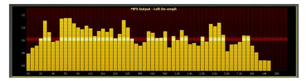
◆ The "FFT Spectrum Analyzer" provides a wealth of information about the audio and composite (MPX) signals throughout the processing chain. Especially useful is the multiplexed composite output display which gives a detailed view of upper and lower sidebands, the pilot, and the RDS signal.
