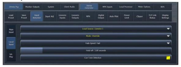
Optionally, Omnia.9sg offers the ability to route an external or "local" audio source into the built-in processor and in turn to the clipper/stereo generator. In addition to the standard internal playback function, this feature provides yet another source of backup audio (plus processing) should both the primary and secondary audio sources fail.
