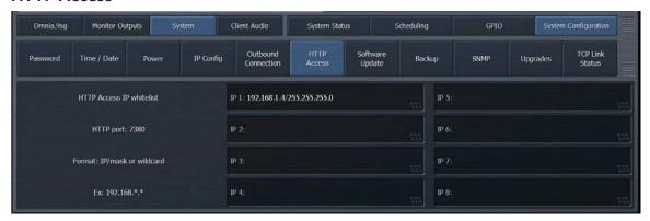
In addition to access via NfRemote, the 9sg has an extensive http remote control interface built in. It is not necessary to configure these settings if you do not plan to use the http interface. This menu ONLY controls access via the remote http interface and does NOT restrict access via NfRemote.
