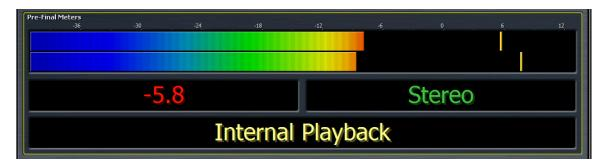
♦ The "Local Processor" display shows input, output, and wideband/multiband meters for the processor used by the internal player and the optional local insertion audio source.
