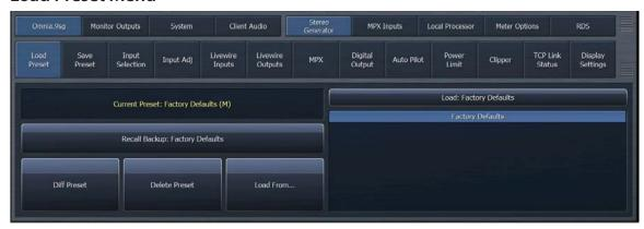
Once you have made changes to the various controls and settings, you will likely want to save those for easy and instant recall. These presets can then be recalled via the "Load Preset" menu. A list of available presets appears on the right side of the screen. Those displayed in white are factory presets. Those displayed in yellow are user presets.
