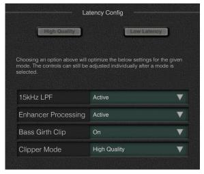
The two option buttons act as "meta-controls": they pre-set the function controls for either maximum processing (all on) or lowest latency (all off).
