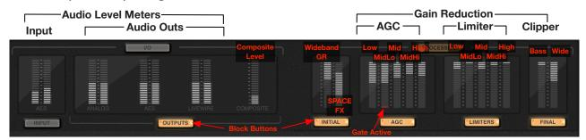
The meter pair on the left shows the selected input's level. You choose whether this will be Analog, AES, or Livewire using the Input Config function button, described below. The next three meter pairs are stereo output level meters. All outputs are active, no matter which input has been selected.
