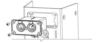
4 - Finally assemble the RDNet plug to the speaker
