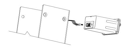
3 - The connector cover is assembled to the RDNet plug accessory to secure and seal the flat cable.
